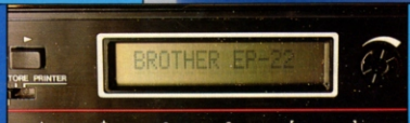
Top right: The EP-22 is slightly smaller than a briefcase, complete with fold-flat handle. Right: The 16-character LCD display.
